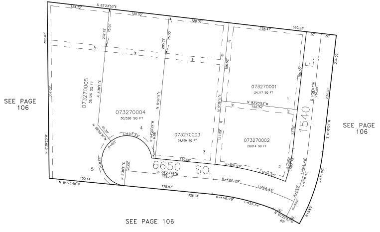
7' UTILITY & DRAINAGE EASEMENTS EACH SIDE OF PROPERTY LINE AS INDICATED BY DASHED LINES OR AS OTHERWISE SHOWN.
